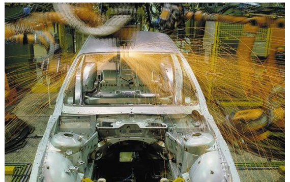
Resistance welding machinery in operation
